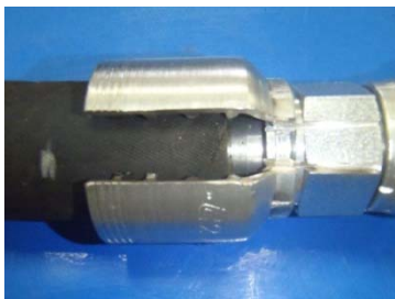
Hose not inserted
